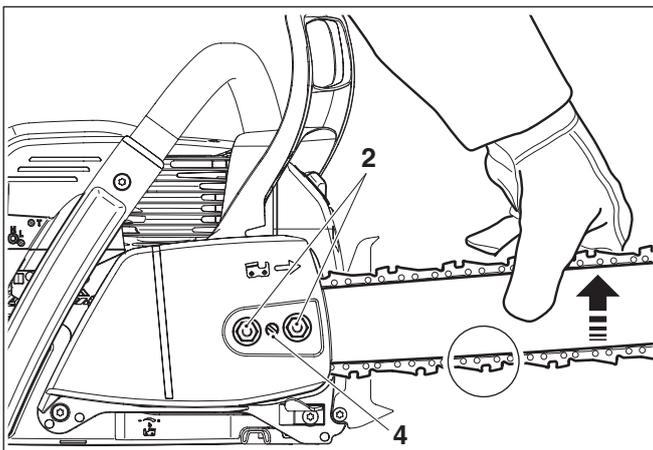
**Tightening the saw chain**
