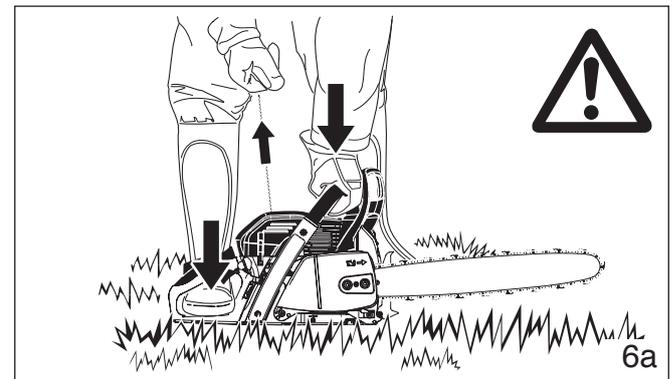
Place the chain saw on firm ground or other solid surface in an open area. Maintain a good balance and secure footing. Place your right foot through the rear handle opening and firmly grasp the front handle with your left hand (fig. 6a).
