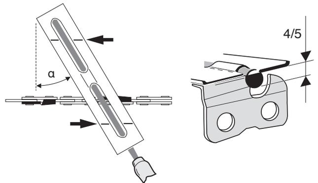
After having sharpened the chain, the height of the depth limiter must be checked by means of a chain gauge. See „Accessories“ for the order number.
