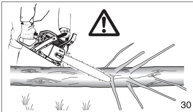
Start limbing by leaving the lower limbs to support the log off the ground (fig. 30). Always cut from the top of the limb.
