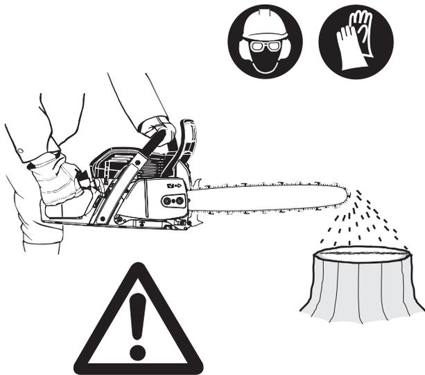
Never work with the chain saw without sufficient chain lubrication. Otherwise the service life of the chain and guide bar will be reduced. Before starting work check the oil level in the tank and the oil feed.
