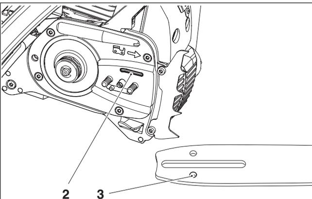
To ensure troublefree operation of the oil pump the oil guide groove at the crank case (2) and the oil inlet bore in the guide bar (3) must be cleaned regularly.
