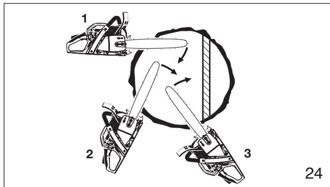
For the sectioning method (fig. 24) make the first cut with the guide bar fanning in toward the hinge. Then, using the bumper spike as a pivot, reposition the saw for the next cut. Avoid repositioning the saw more than necessary.
