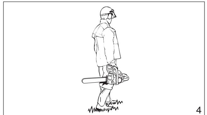
**By hand:** When carrying your saw by hand, the engine must be stopped and the saw must be in the proper position.
