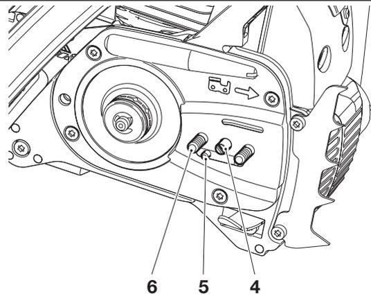
Put on the guide bar (7). Make sure that the pin (5) of the chain tensioner engages in the hole in the guide bar.
