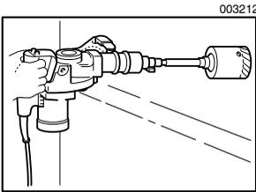
Rotate the change lever to the  $\top$  position. Rest the core bit on the concrete and turn the tool on. Once the core bit has cut a shallow groove into the concrete, rotate the change lever to the  $\text{BT}$  position and resume drilling.
