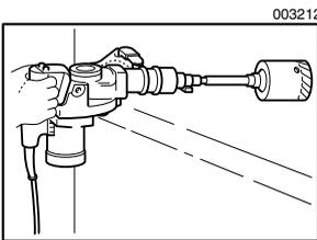
Rest the core bit on the concrete and turn the tool on. Once the core bit has cut a shallow groove into the concrete, remove the center bit. Then resume drilling.
