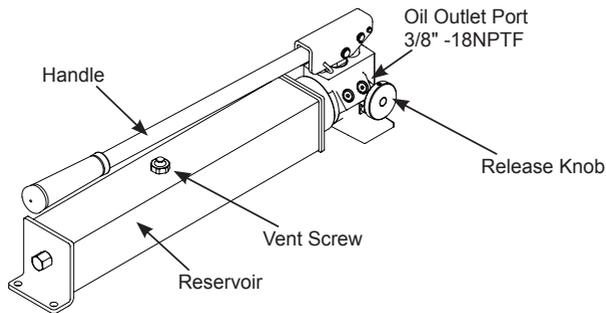
Figure 2 - Model P2001-5K Components
