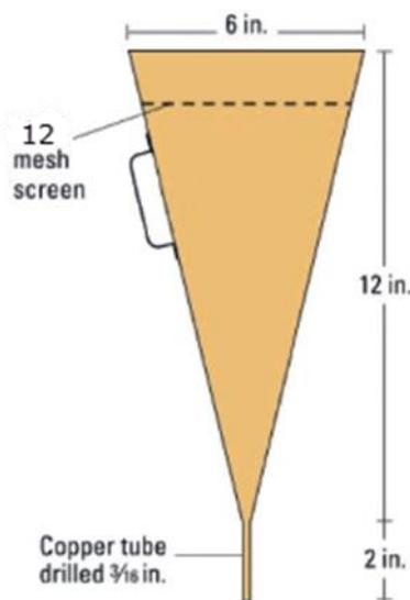
*The Marsh Funnel is precision-made to outflow one quart of water at  $70 \pm 5^\circ\text{F}$  in  $26 \pm 0.5$  seconds.*
